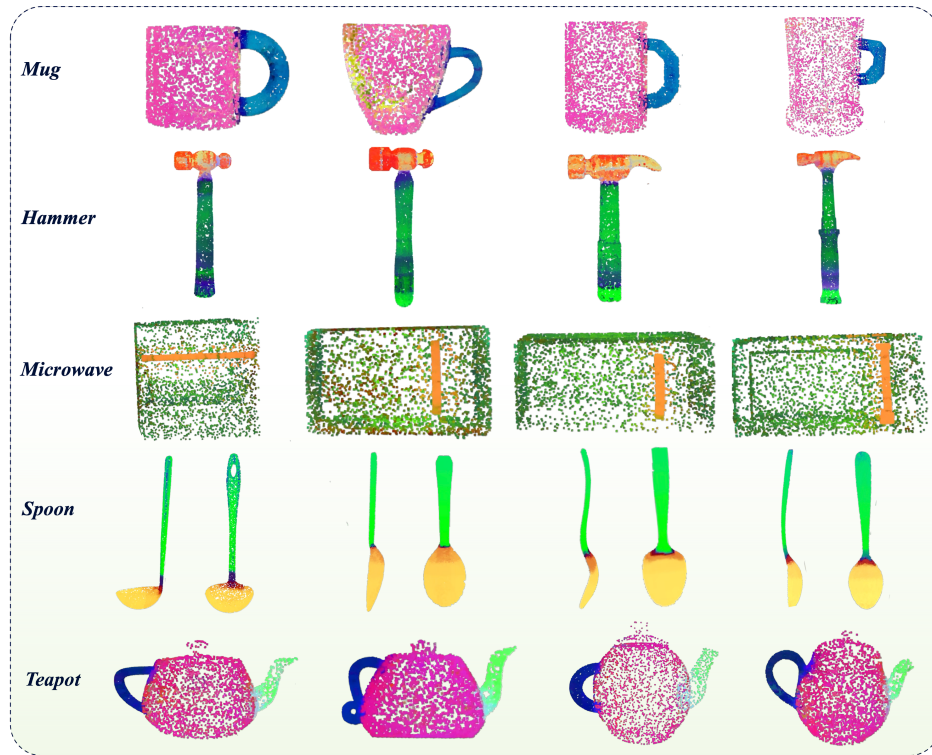
Figure 8: Additional qualitative visualizations of queried semantic embeddings on mugs, hammers, microwaves, spoons, and teapots. Similar colors indicate similar embedding responses after RGB projection, highlighting consistent part-aware patterns across object instances.
