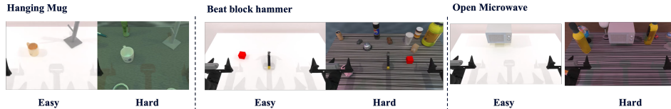
Figure 5: Simulation task examples used in our evaluation. These tasks require localizing functional object parts, such as mug handles, hammer heads, articulated handles, and placement regions, to complete object-centric manipulation.
